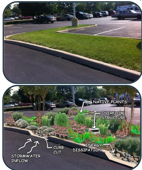
Figure 7.2 Bioretention: Before and After Parking Lot Island.
